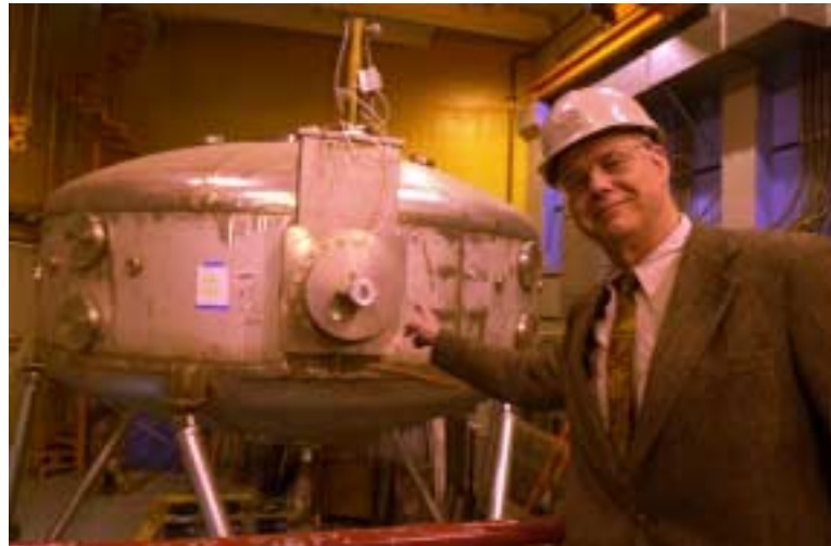
Miklos Porkolab, Director of MIT's Plasma Science and Fusion Center, stands next to the Center's Levitated Dipole Experiment, a new approach to fusion.
