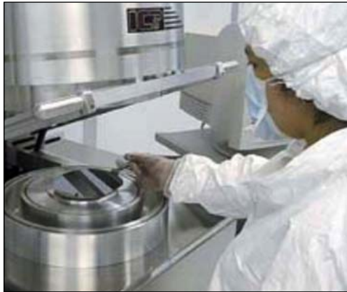
A technician prepares a plasma etcher, placing the wafer on the lower metal plate. In a large commercial manufacturing environment, the wafers are handled by robots, not humans.
