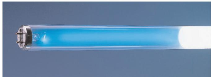
**The plasma in a fluorescent lamp produces ultraviolet light that is converted to visible light by the phosphor coating on the wall. This photo shows a lamp with part of the white phosphor coating removed to reveal the blue plasma glow inside.**
