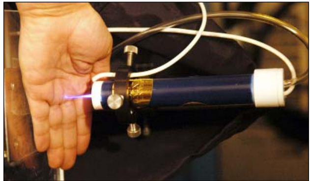
A cold plasma can contact skin without harming it, making it ideal for disinfecting wounds.
